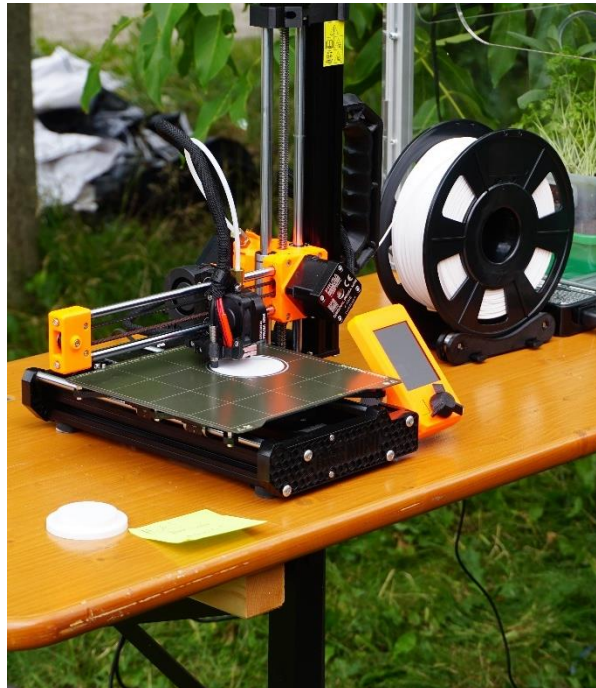
Figure 55: 3D printing the feet.
