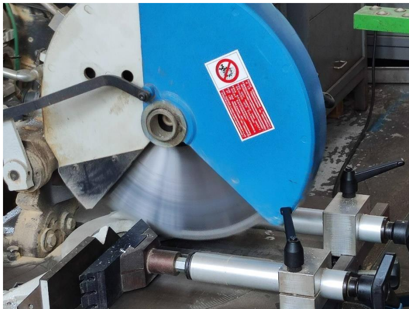
Figure 46: Sawing the T-slotted aluminum profiles.
