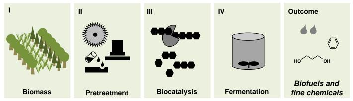
Schematic diagram depicting conversion steps to produce second-generation biofuels and platform chemicals from plant-derived lignocellulosic biomass.
